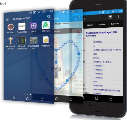
Cryptojacking in an innocent app and the resulting performance hit on a Sony Xperia M2
